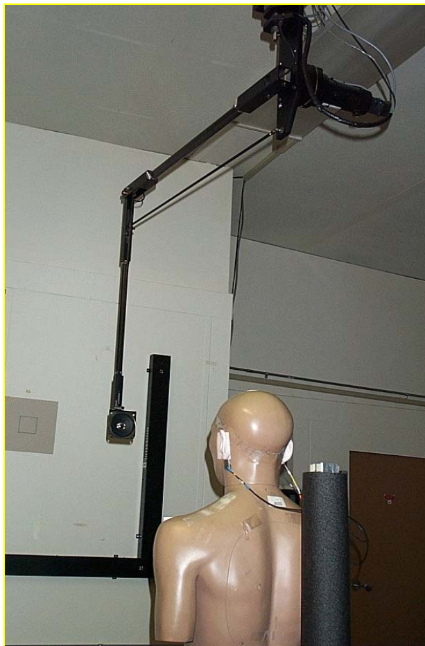
Figure 1 – The RoboArm 360 system. The computer-controlled robotic arm can place the loudspeaker to 1° precision.
